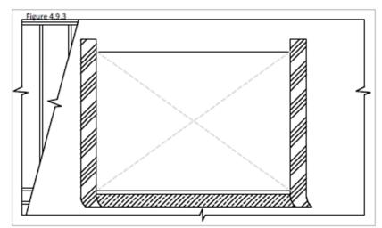
point to assure contact with the backside (interior) of the mounting flange. Apply sealant in line with the pre-punched holes or slots on the mounting flanges.
