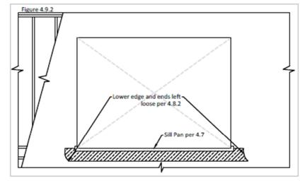
ends of the flashing should be secured to prevent curling or contamination of the adhesive surface prior to installing the exterior facade.
