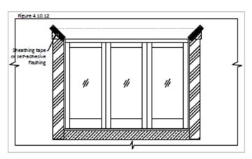
**4.10.12** Apply a piece of sheathing tape or self-adhering flashing over the entire diagonal cut made in the WRB during step 4.9.4 and press firmly assuring contact between the WRB and the tape or flashing as in Figure 4.10.12.
