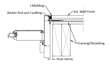
exterior wall surface (siding, stucco, etc.) then apply sealant per the sealant manufacturer's recommendations along with reference to the methods set forth in ASTM E2112.
